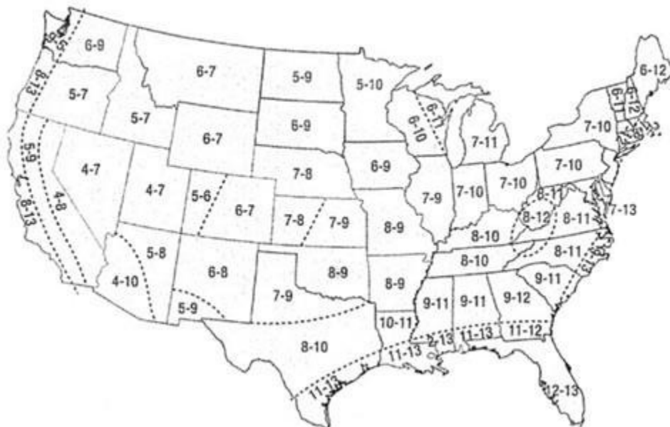
Moisture Content Map, from the US Department of Agriculture, Forest Products Laboratory
